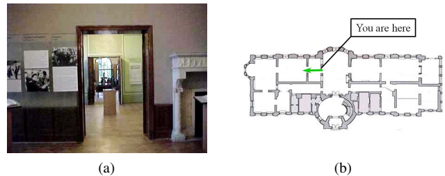
Figure 1: Our system takes a video stream and a floor-plan, and outputs the position and orientation of the current frame in the floor-plan.
